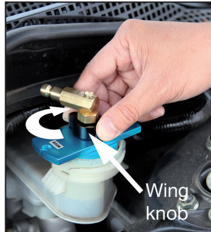
Fig. 5: Tighten wing knob to expand o-ring
