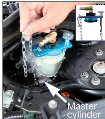
Fig. 6: Install chain around master cylinder to retain adapter
