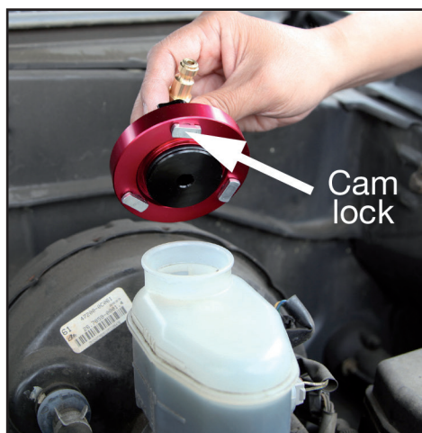
Fig. 8: Verify cam locks are turned as shown
