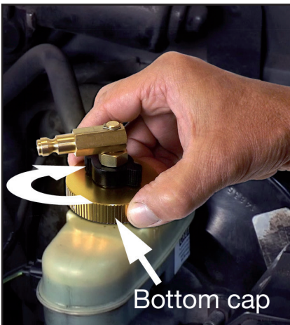
Fig. 2: Select and install correct adapter
