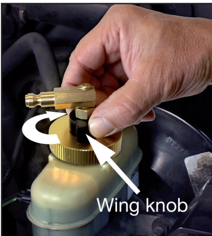
Fig. 3: Tighten wing-knob to expand o-ring
