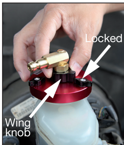
Fig. 9: Turn cam locks to engage reservoir and tighten wing knob
